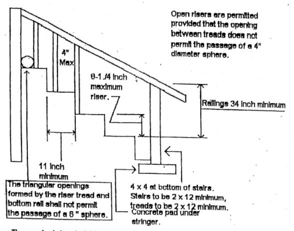
The greatest riser height within any flight of stairs shall not exceed the smallest by more than 3/8 Inch.
