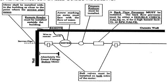
Diagram for Water Meter/Remote Installation
